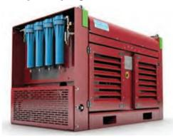
This unit takes instrument air available on the rig through air separation membranes and delivers high purity nitrogen (98 per cent) at high pressure (5000 psi).
