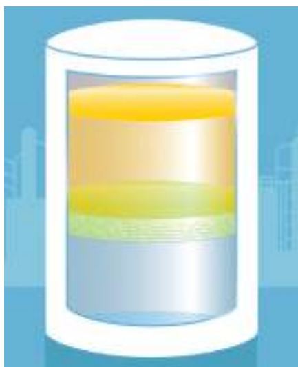
Figure 1: Multiphase level often includes hydrocarbon at the top, emulsion (rag layer) in the middle and water at the bottom.
