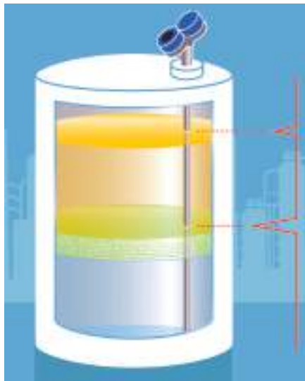
Figure 2: GWR with signal reflections down probe.
