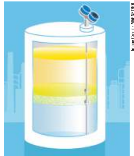
Figure 3: Direct-insertion magnetostrictive transmitter measuring emulsion layer.
