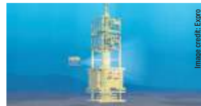
Expro's IRS solution will safely establish and maintain well access through riser to surface operations.
