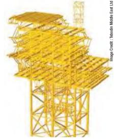
A SACS model of a complex offshore platform.
