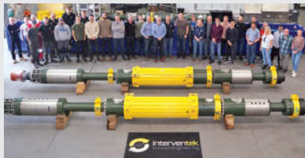
Interventek's new API 17G qualified subsea landing string, pictured with some of the team involved in its commercialisation.
