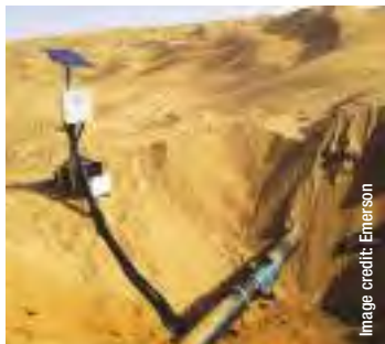
Roxar FSM Log 48 Area Corrosion Monitor detects both localised and generalised corrosion.
