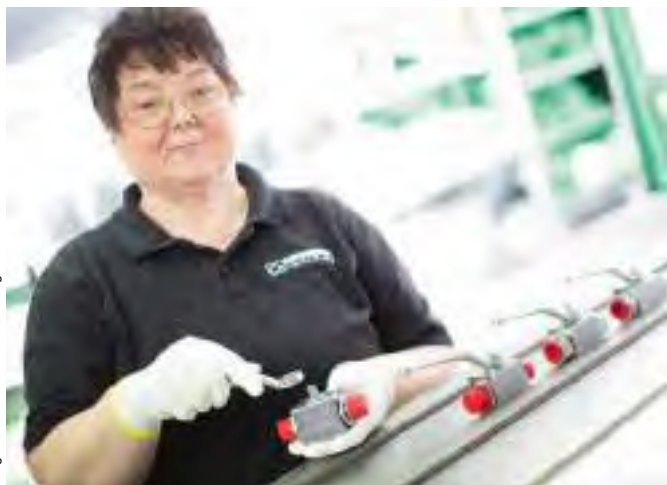
The final installation of two-way valves takes place in the Stauff Logistics Centre.
