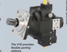
a focus on high-performance machines. Due to the V16's innovative differential piston control system, along with a three-way valve and best-in-class displacement ratio (5.5:1), the V16 offers smooth and precise control. The patented spherical piston design with laminated piston rings provides a high shaft speed capability, up to 30% higher than competitors. In combination with the high-pressure level, up to 550 bar, the V16 offers enhanced performance
