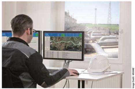
An E-RTTM leak detection system creates a virtual image of a pipeline based on real measured data.
