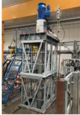
Amarinth API 610 VS4 vertical pump undergoing final test before
