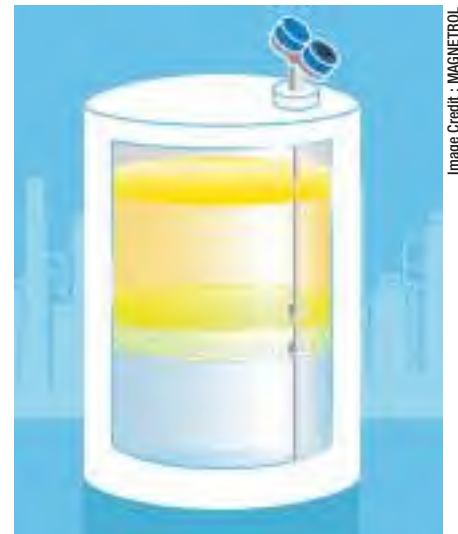
Figure 3: Direct-insertion magnetostrictive transmitter measuring emulsion layer.
