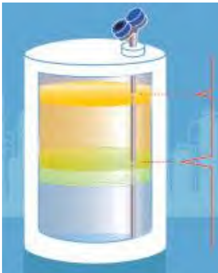
Figure 2: GWR with signal reflections down probe.
