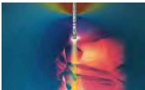
The IriSphere service multifrequency transmitters and multireceiver BHA provide continuous resistivity that detects formation features far ahead of the drill bit.
