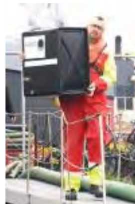
Oil spill responder carrying a 25m T-Fence cartridge
