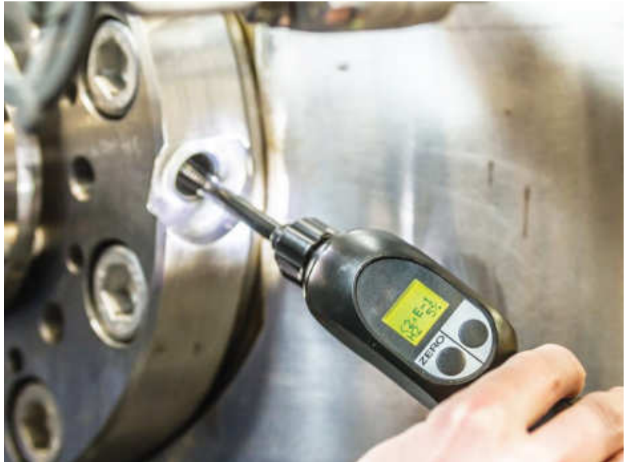
With its material suitability testing, Hartmann Valves offers a test enabling checks of existing valves for application with hydrogen.
