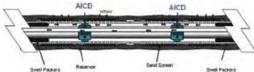
Figure 3: Retrofit AICD completion in existing standalone screen with the production flow paths
