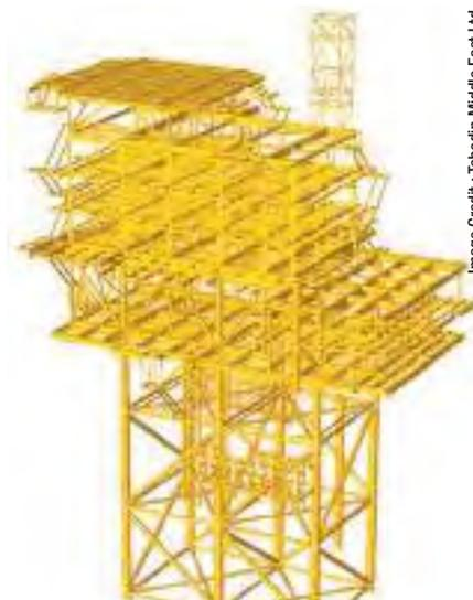
*A SACS model of a complex offshore platform.*
