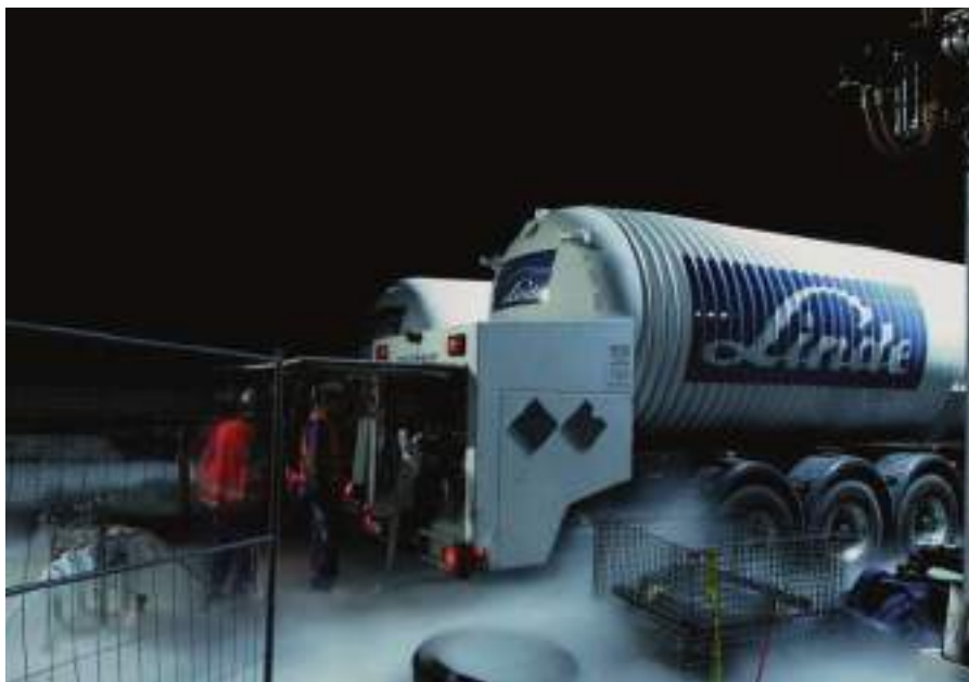
Liquid nitrogen is used for ‘dry fracturing’ – a fracturing process that has eliminated many of the problems associated with hydrofracturing
