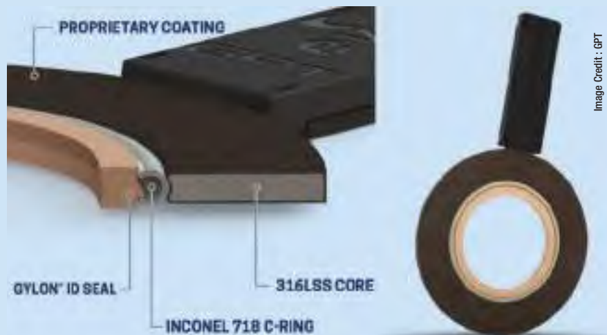
EVOLUTION, the fully-coated isolation gasket.
