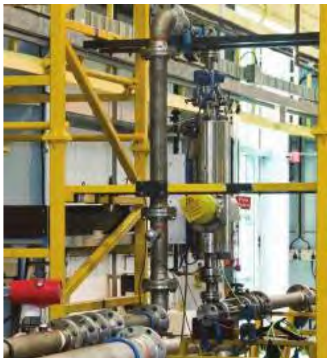
Multiphase meter undergoing testing at NEL's multiphase flow measurement facility
