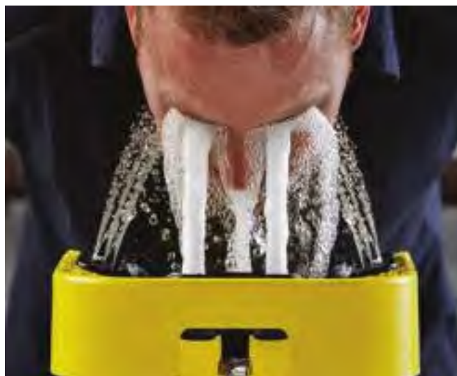
The ABS plastic basin is fitted with aerated sprays for eyewash comfort and innovative face pads for full face cleansing while the water flow is activated by a large stainless steel push handle with a stay-open valve for hands-free operation. (Photo: Empteezy)
