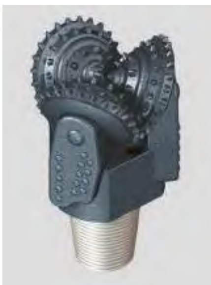
Tricone bits are protected by using abrasion-resistant and slurry erosion resistant carbide materials PTA and laser cladding based materials or oxy-acetylene hard face welding products
