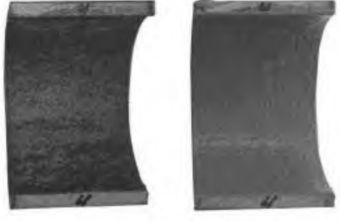
Tubular part before and after with MAOK-GT® coating
