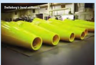
its termination point. The bending stiffener is also designed to transfer load via a suitable path from flexible pipe to the fixed structure. Its conical shape provides a gradual transition in stiffness, hence preventing over bending at the termination
