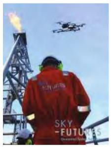
UAVs (unmanned aerial vehicles) are able to capture data from the structure, in HD video, stills and thermal formats
