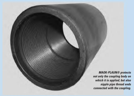
The MAOK-PLAUN® coating test was done on BUTTRESS screw joints of API Spec5CT standard casing pipes. The BUTTRESS joint with the coating of casing pipe with 146 in diametre of strength group N80 during tests for gas tightness withstood a pressure of 600kgs/sg cm for 65 hours. Consequently, the BUTTRESS screw joint of strength group H40 withstood the recommended testing pressure of 300kgs/sq cm, the company said.
