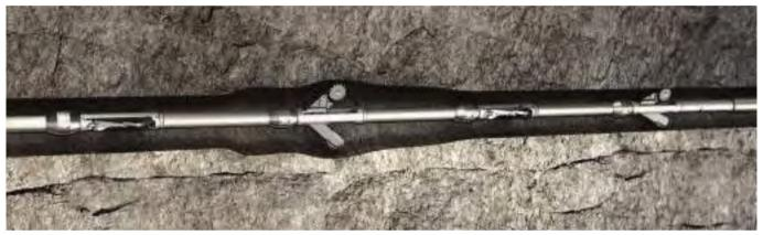
Figure 1. UltraTRAC all-terrain tractor delivers more than twice the efficiency of conventional drill pipe conveyance methods in openhole laterals; the tandem configuration of the tractor allows negotiating abrupt changes in borehole geometry (Image courtesy of Schlumberger)
