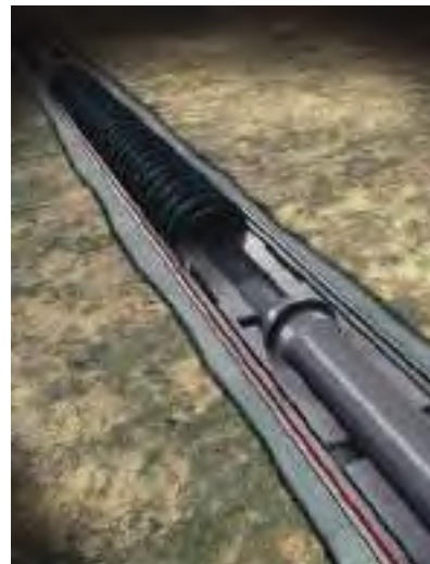
The STP lubricates and keeps sand out of the barrel/plunger interface area (Photo: Weatherford International)
