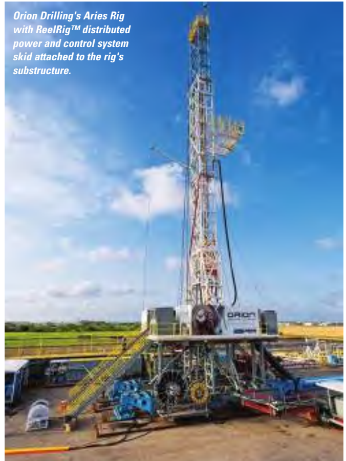
Fig. 3: ReelRig™ power cable and communication cable spooling skid
