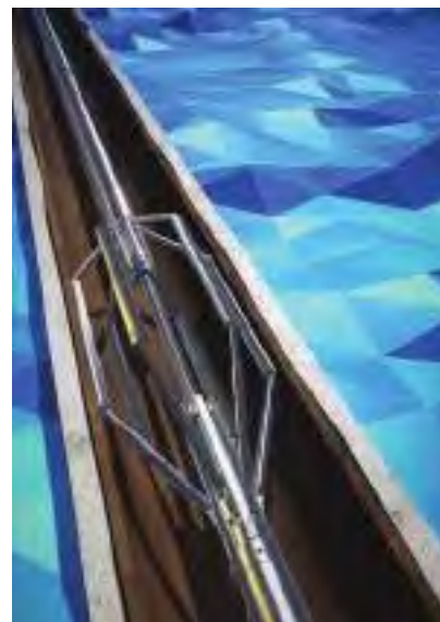
Integrity eXplorer utilises electromagnetic-acoustic sensors
