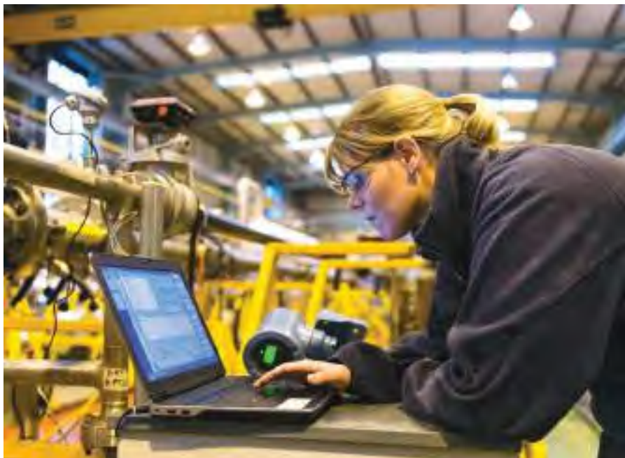
Meter calibration in NEL's flow measurement facility
