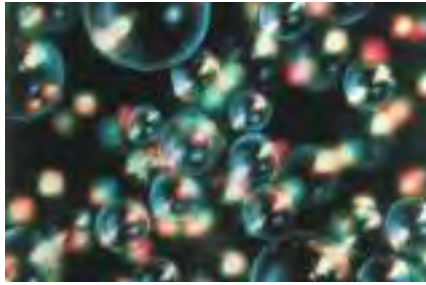
3M's glass bubbles are used as a density reducing agent
