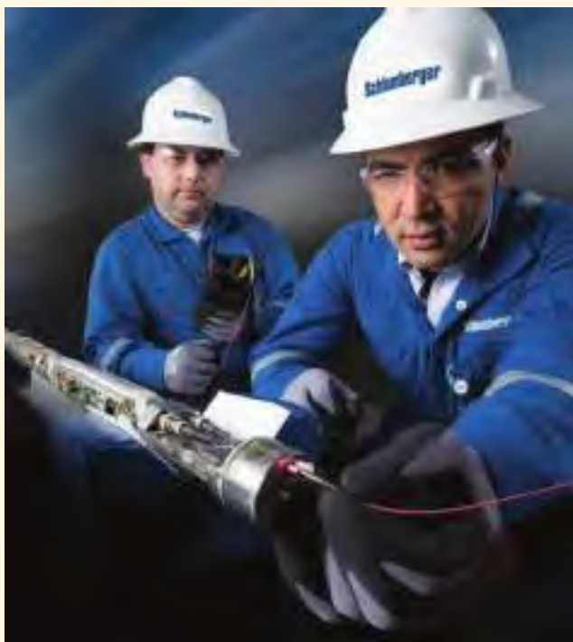
During lab testing, the ACTIVE OptiFIRE system successfully actuated more than 40 simulated detonators at the full temperature rating of 175°C
