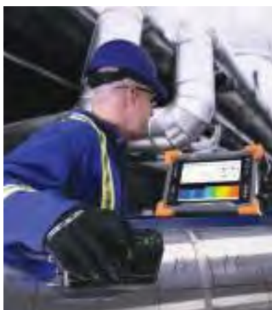
The Eddyfi Lyft™ is an inspection tool for identifying corrosion under insulation (CUI)
